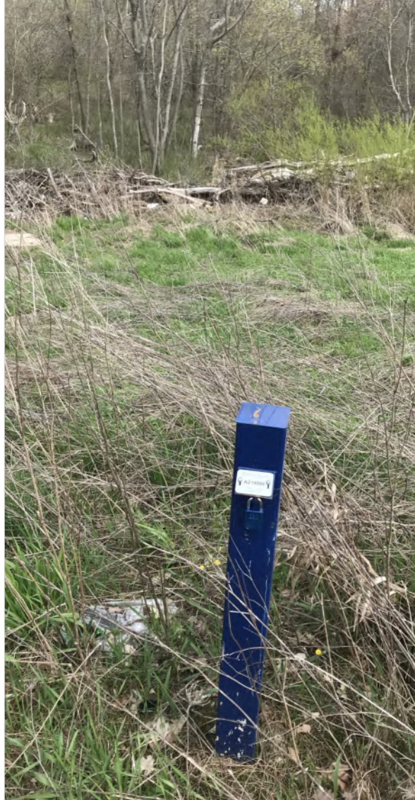
Photo 21: view of monitoring well MW101.
