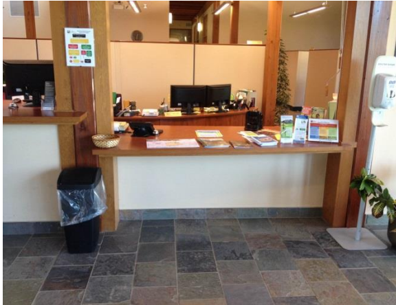
Low customer service counter can accommodate users of mobility aids
